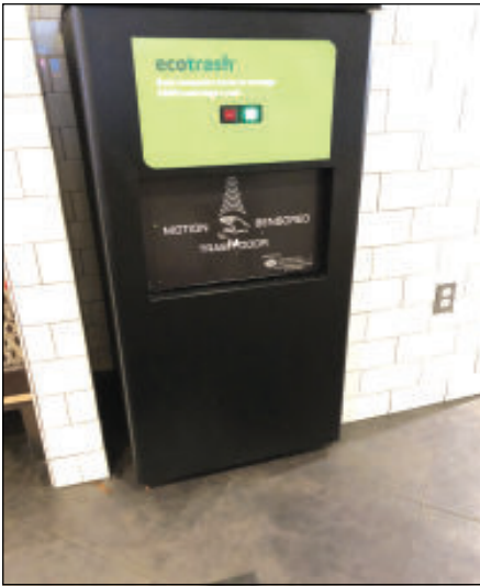
Image. Ecotrash is a type of automatic compacting receptacle at a fast food restaurant, 'Chick fill A', downtown Chicago. The compactor is great for small incremental trash deposits. The trash door is 'motion sensed' – it pulls in the trash tray inside. Every year each compactor saves 6960 trash bags, reducing plastic use ". A compactor can hold 300 gallons (40.1 cft) of compressed trash. On right: common kitchen trash bag with strap.
